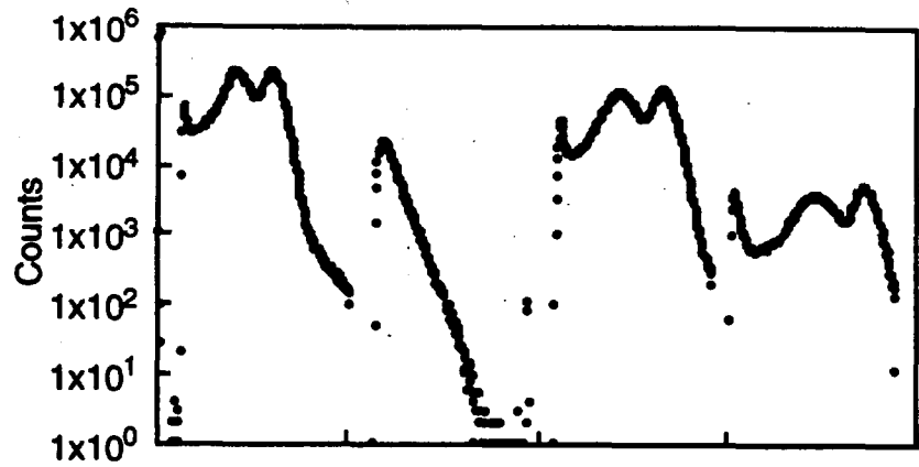
Figure 2.11. Data from a fission chamber in Big Ten. Four spectra are acquired and displayed simultaneously. The second spectrum above is from the blank barrel.
