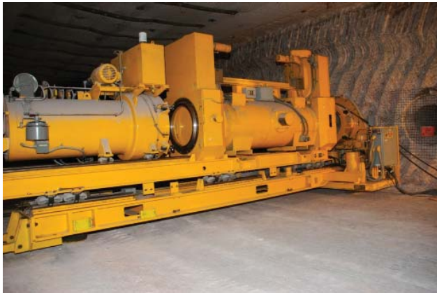
Horizontal Emplacement and Retrieval Equipment (HERE) for Emplacing RH Canisters in the Underground
