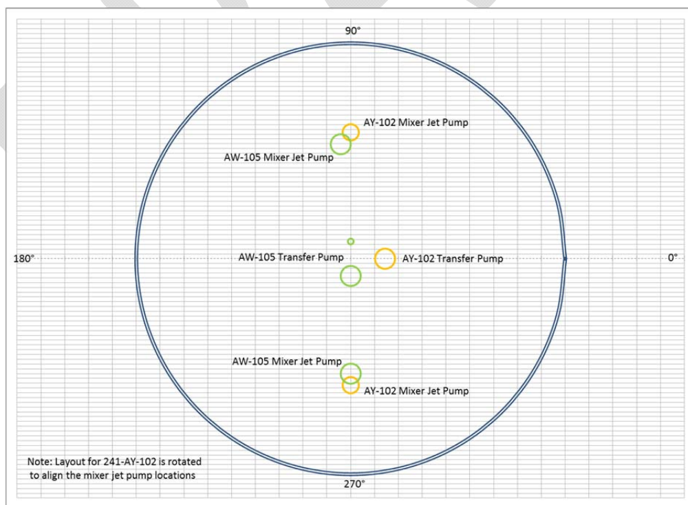
Figure 3-2: Comparison of Equipment Layout for 241-AY-102 and 241-AW-105
