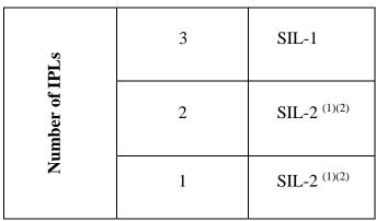
Figure B.2-1: SIL Determination Methodology
