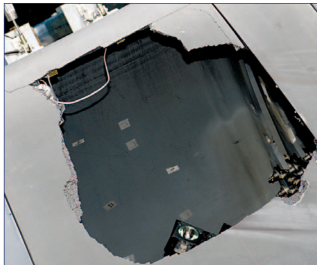
Figure 3.8-9. The large impact hole in Panel 8 from the final test.
