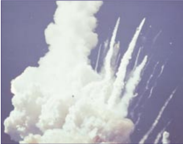
Figure 1.5-1. the Space Shuttle Challenger was lost during ascent on January 28, 1986, when an O-ring and seal in the left Solid Rocket Booster failed.
